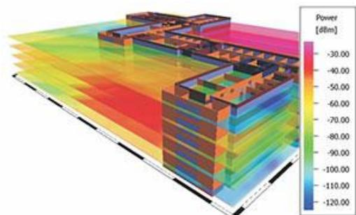
Depending on the application, **CellTrace™** offers static, Monte-Carlo, and dynamic network simulators. It also allows for the planning of coverage and capacity as well as network simulations.
