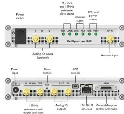
**CellSpectrum™ 1000** does not compete with traditional spectrum analyzers, filling instead a gap between field spectrum analyzers and laboratory spectrum analyzers.
